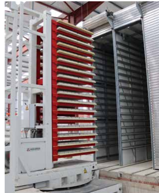
Finger cart system load capacities (8.5t, 14t, 24t)
